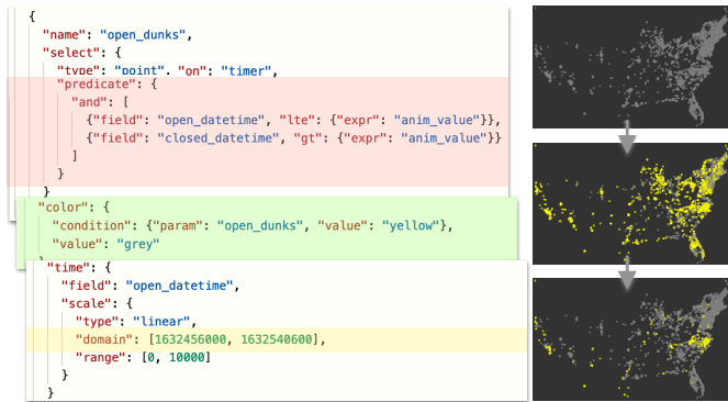
Fig. 3. Animation of Dunkin’ Donuts stores’ opening and closing times. With a custom domain and predicate, the animation advances through 24 hours at a constant rate and conditionally colors each store if the current time is between the store’s open and close times.
