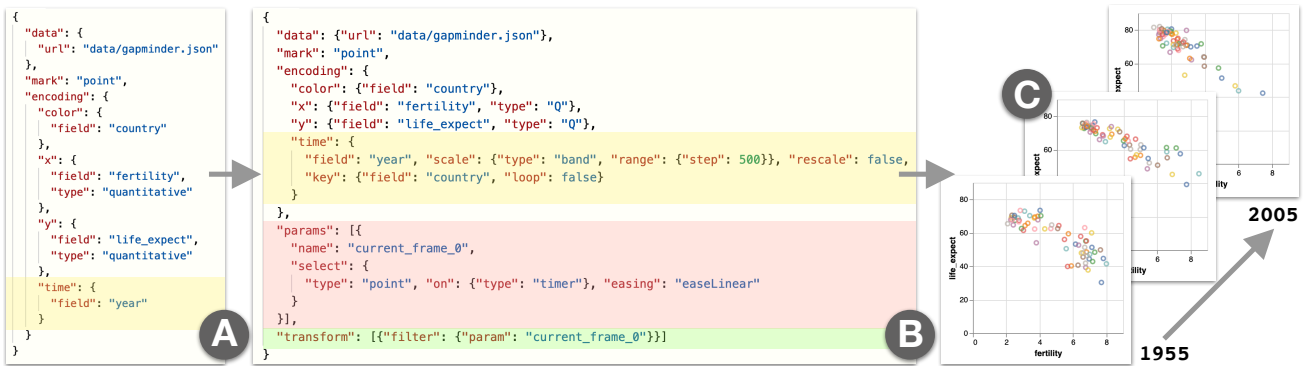
Fig. 2. Animated Vega-Lite specification of the influential Gapminder animation [34]. (A) A minimal specification using only time encoding. (B) The same specification elaborated to show default encoding properties and a default selection. (C) Selected keyframes from the resulting animation.
