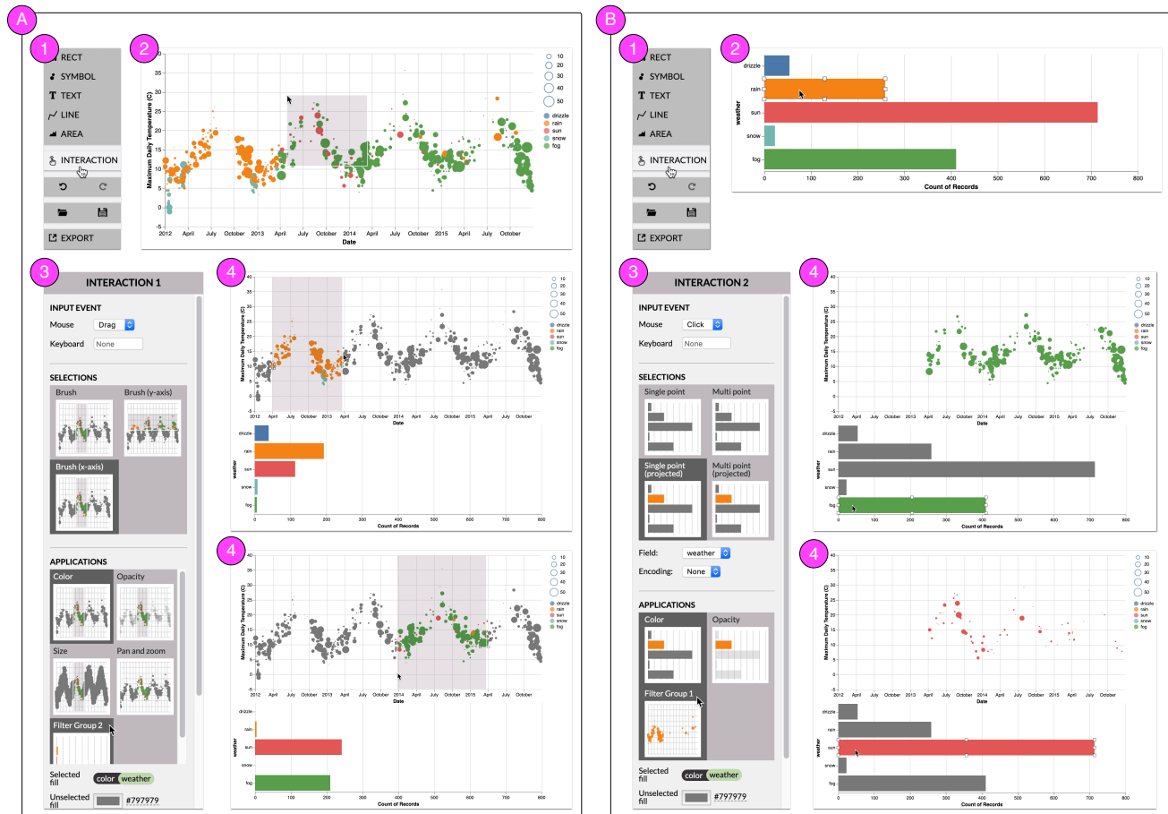
Fig. 2. The process of creating the interactive visualization in Fig. 1. (a) Demonstrating a horizontal brush that colors selected points in the scatterplot and re-aggregates the histogram. (b) Demonstrating a click interaction that colors the selected bar and filters the scatterplot via the weather field.
